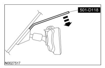
4. Release the mirror mount from the windshield bracket by pulling the Mirror Remover and mirror down and away from the windshield.
